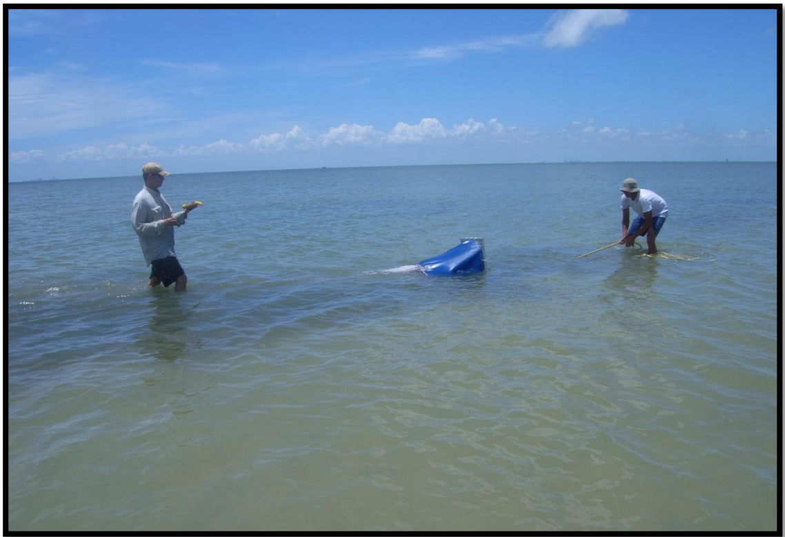
Figure 4. Photograph of the epibenthic sled being towed through a small seagrass patch within a highly fragmented network. The sled's path is then recorded using a Trimble.
